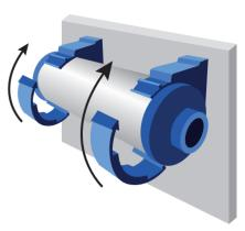
4. Close the brackets so the filter is secured.
