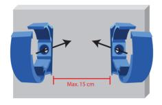
2. Mount the brackets to a wall or wooden plate. NOTICE: The distance between the bracket can only be 15 cm.
